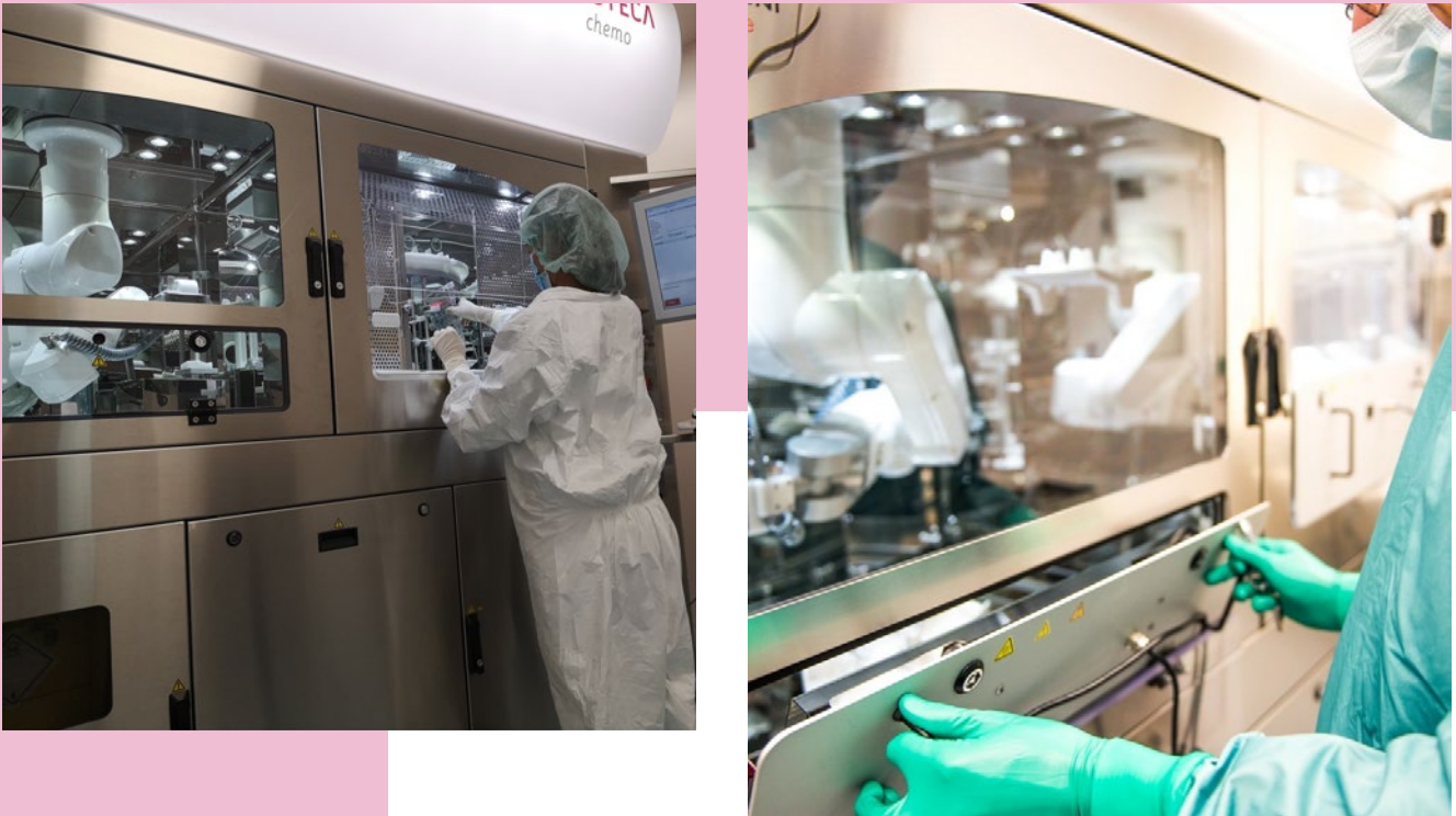
Figure 10-3: Preparation of infusion bags with HMPs in an automated robotic system at the Amsterdam UMC, The Netherlands. Operators are wearing PPE.
